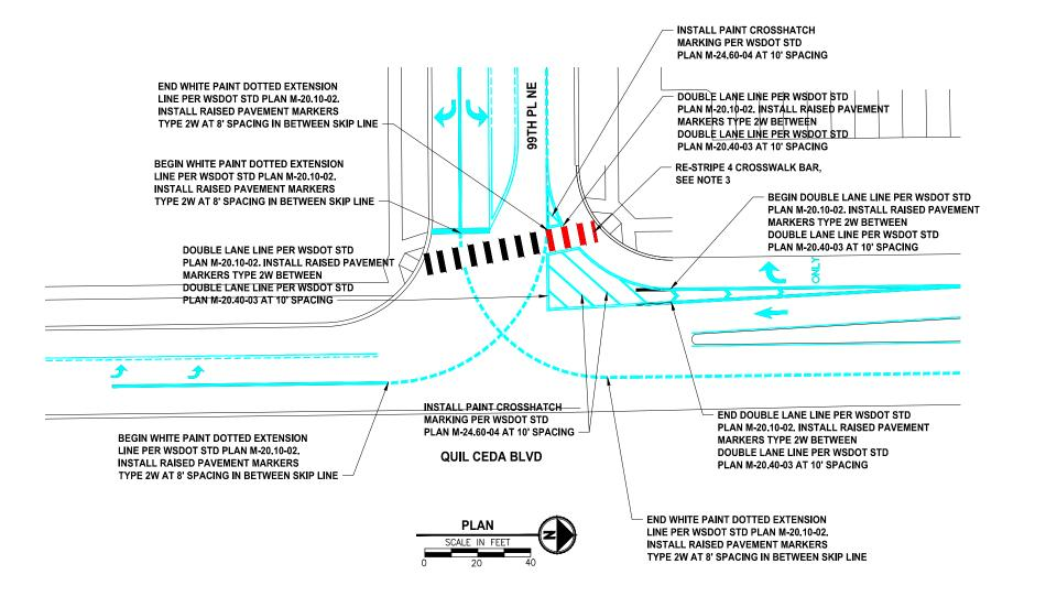
PAVEMENT SURFACE SHALL BE PREPARED FOR THE NEW MARKINGS. INCLUDING COMPLETE REMOVAL OF THE OLD PAVEMENT MARKING PER SECTION 8-22 OF THE WSDOT STANDARD SPECIFICATION.
